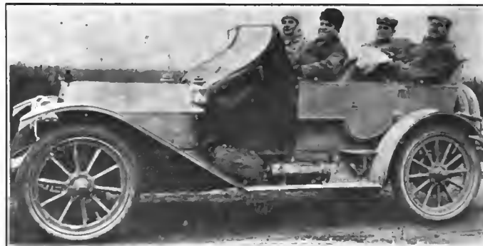
Benzine test on a Fal-Car fitted with a Rayfield carbureter made to determine the feasibility of using heavy hydrocarbon fuel instead of gasoline proper
